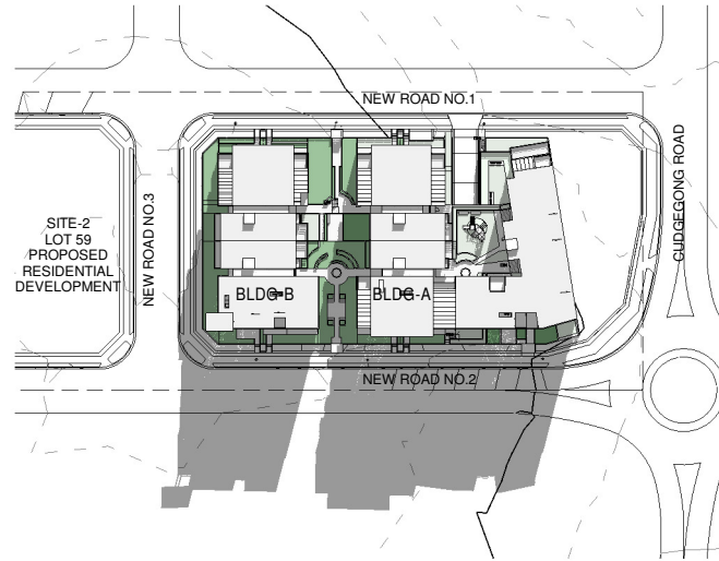
SHADOW DIAGRAM WINTER SOLSTICE JUNE 21 1:00 PM
